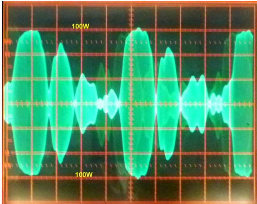
Figure 4: SSB RF envelope at 100W PEP. Note ALC compression on voice peaks.
